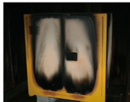
▲ Cabinet fire exposure test conducted by FM Approvals.
